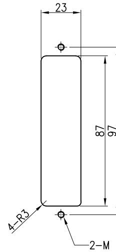
Panel Drilling Dimension
